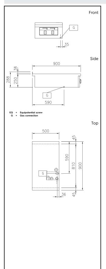
Gas Gas Power: 20 kW Gas Type Option: Gas Inlet: 1/2" **Key Information:** External dimensions, Width: 500 mm 900 mm External dimensions, Depth: External dimensions, Height: 250 mm Net weight: 41 kg Configuration: One-Side Operated;Top Front Burners Power: ISO 9001; ISO 14001 - kW **Back Burners Power:** 10 - 0 kW **Back Burners Dimension -**Ø 70 Front Burners Dimension -Ø 70
